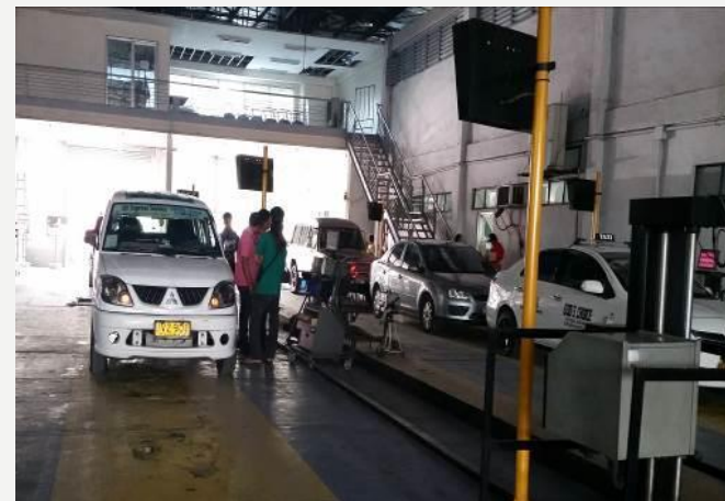
Equipment for checking brakes and sideslip
