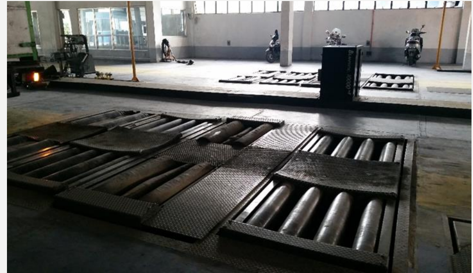
Equipment for checking brakes and sideslip
