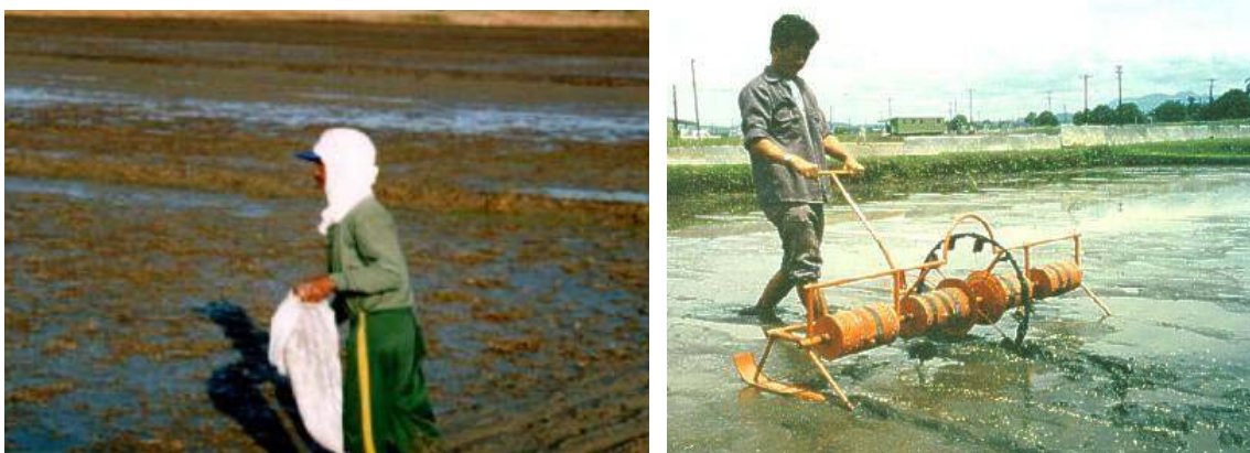
Fig. __. The IRRI drum seeder facilitates wet seeding in neat rows with less seeds than broadcast seeding.
