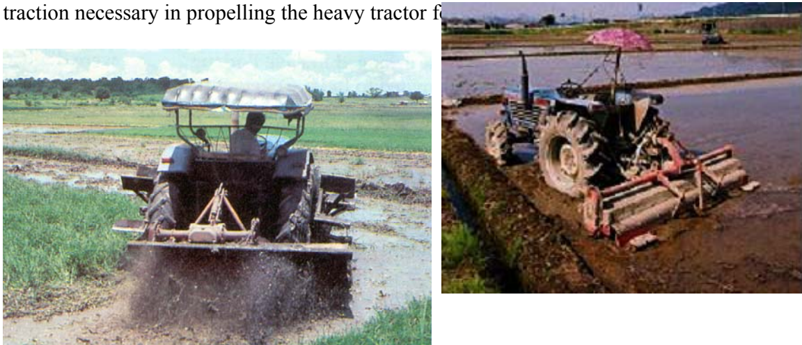
Fig. __. Big four-wheel tractors with rotavating attachment preparing flooded rice fields.
