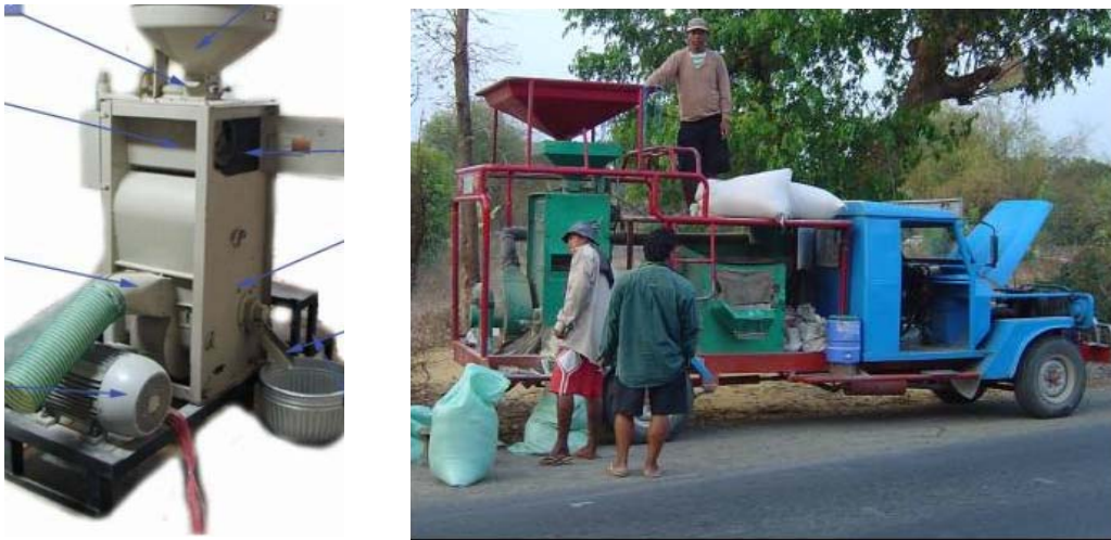
Fig. __. Single-pass rubber roll rice mills as stationary units in village/town centers or mounted behind locally assembled jeep provide milling services in the villages.
