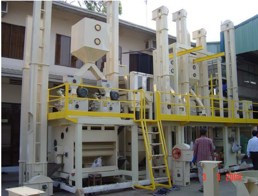
Fig. __. Modern rice mill systems employ multiple passes of grains through different mill components to maximize recovery and whole grains output.
