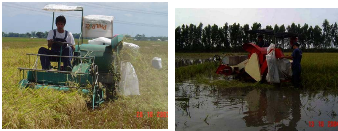
Fig _. This small and lightweight rice combine is more appropriate for small wet fields in the Philippines than the big and sophisticated imported combines.
