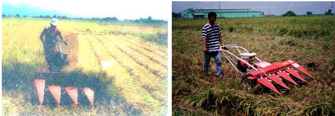
Fig. __. The IRRI reaper can harvest 2.4 ha/d but its popularity was overtaken in the late 1980s with an imported harvester from Japan.
