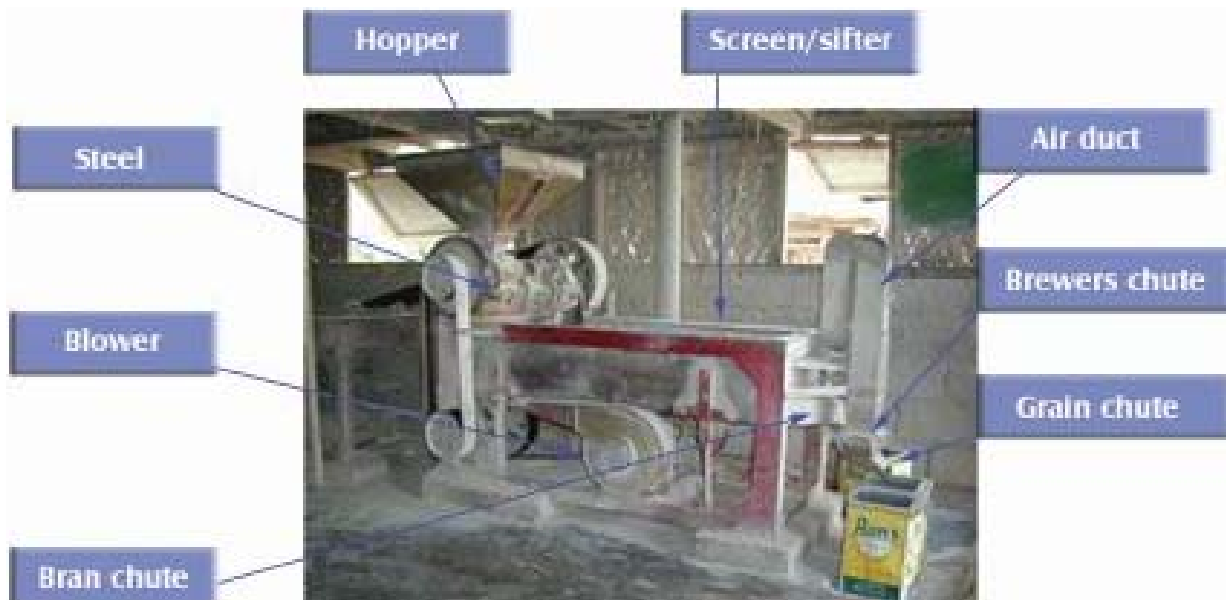
Fig. __. Village kiskisans provide milling services in the villages for a long time until its use was discouraged by the government due to its low recovery.
