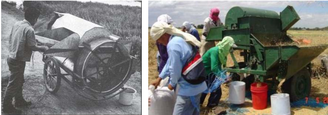
Fig. __. IRRI axial-flow thresher released by IRRI in early 1970s and commercial model at present.
